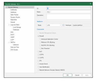
The left side of the dialog box contains the sections of the Security Gateway settings. The right side contains the respective parameters.
