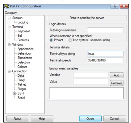
**5.** In the **Terminal-type string** text box of the **Terminal details** group box, enter **Linux**.
