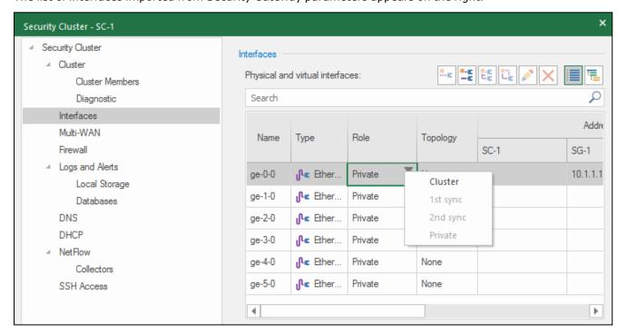
2. Select the role for each interface of the security cluster and modify the other parameters if necessary. Specify IP addresses for external and internal interfaces of the security cluster. IP addresses of the security cluster virtual interfaces and its members must be in the same subnet for each interface.
