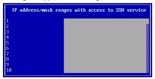
**4.** Type the required IP address of a remote host in the form of **xxx.xxx.xxx.xxx.xxx.xxx.xxx** or a subnetwork with its prefix the following way: **xxx.xxx.xxx.xxx**[/xx]. Press <**Enter**>.
